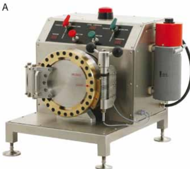
Figure 3: Pyrolyser-Trio combustion furnace for extraction of total tritium
